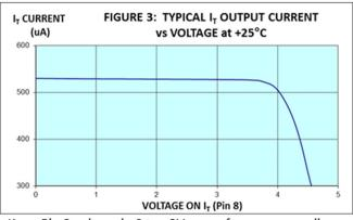
Keep Pin 8 voltage in 0 to +3V range for proper readings.
